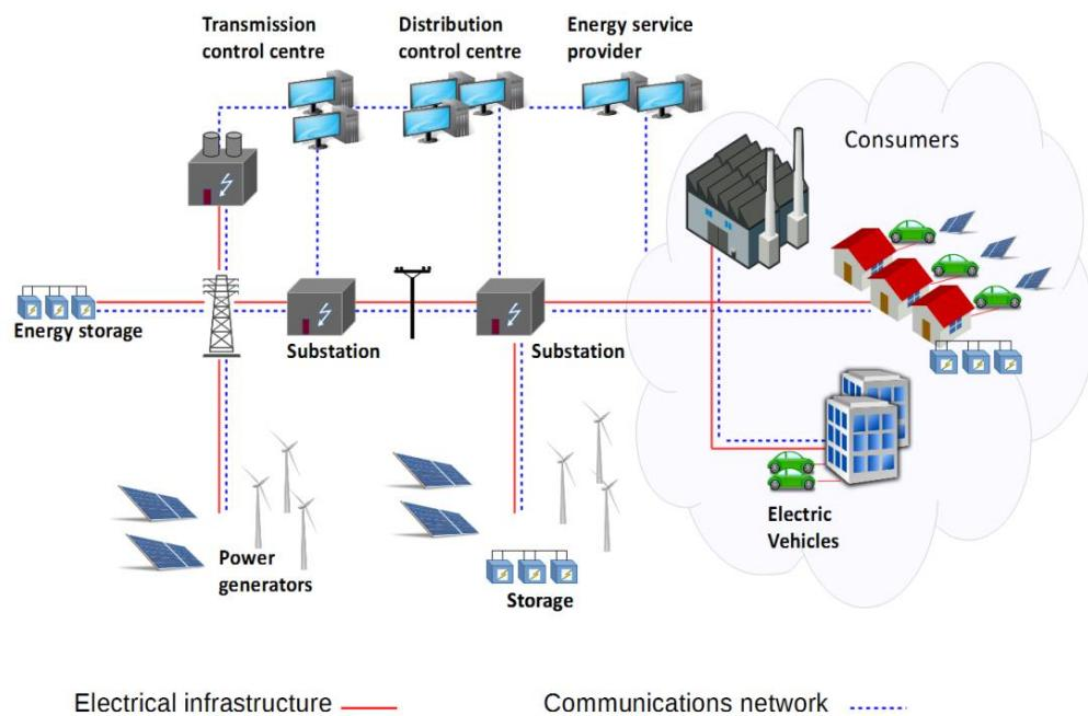
Each type of DER system has its own unique characteristics but, in general, they can be treated as a small to medium-sized sources of electric power. Electric Vehicles (EVs) can sometimes act as DER systems, however as they have different purposes, they are usually identified as a separate entity from the rest of DER systems.
